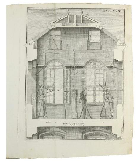
Culminatorium, for the observation of the meridian Marinoni's passages, wall quadrant, the Quadrans ampliatus, the position micrometer with its screws, a camera obscura, and pendulum clocks ("for his observations he used 5 pendulum clocks; two he had obtained from G. Graham and then had 2 similar clocks built in Vienna. The 5th clock had been built by Faucheuer in Paris in 1736 and had been provided with a dial to indicate the mean time and the equation of time", see Zinner).
